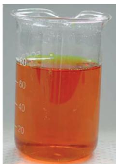
Figure 2: Active in purified water at 60 °C. The dissolution was incomplete.
