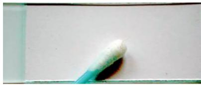
Figure 8: Exposure of test substrate made from borosilicate glass to a solution of 1 % (v/v) formulated cleaner at 60 °C. After rinsing the substrate was completely dry before swabbing.
