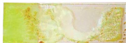
Figure 4: Active ingredient in organic solvent. Preparation borosilicate glass and dried down. Before cleaning.
