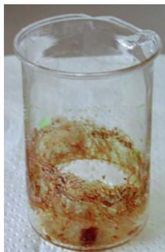
Figure 1: Example if using organic solvent during cleaning. Residue of the active remains (source of all figures: Borer Chemie).
