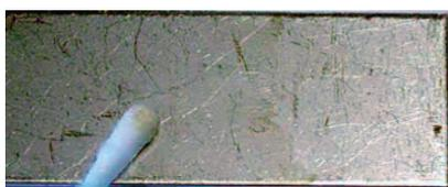
Figure 7: Exposure of test substrate made from stainless steel to purified water at 60 °C. After rinsing the substrate was completely dry before swabbing.
