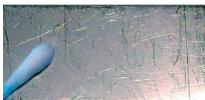
Figure 9: Exposure of test substrate made from stainless steel to a solution of 1 % (v/v) formulated cleaner at 60 °C. After rinsing the substrate was completely dry before swabbing.
