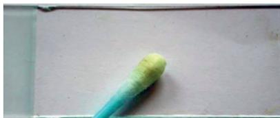
Figure 6: Exposure of test substrate made from borosilicate glass to purified water at 60 °C. After rinsing the substrate was completely dry before swabbing.
