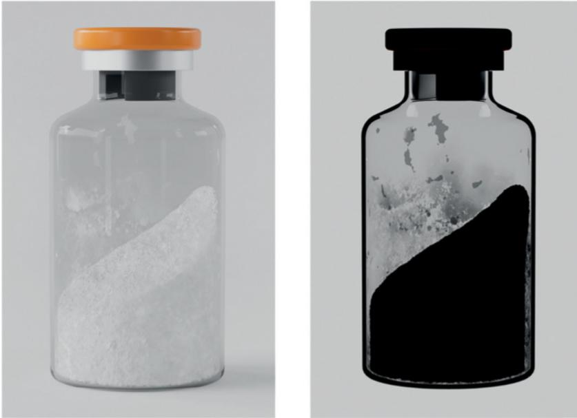
**Figure 8: Structural damage in the lyo cake becomes clearly recognizable as well.**
