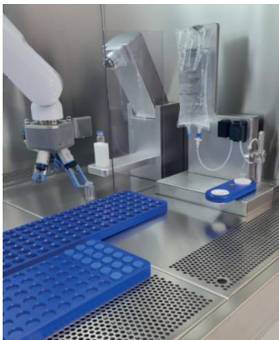
**Figure 2:** The triple gripper transfers and places the vials.
