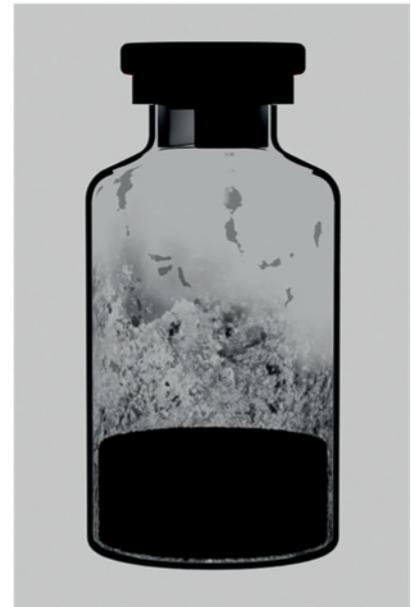
*Figure 7: Product adhesions on the vial walls become more clearly visible when inspected with transmitted light.*
