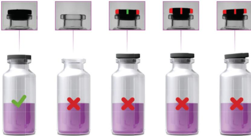
**Figure 3:** Under cleanroom conditions, it is checked whether the important sealing elements are present and correctly seated.
