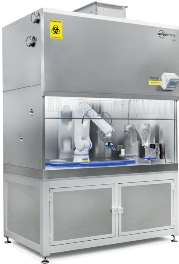
**Figure 1:** The Safety Workbench with an integrated robot removes the vials from a magazine, transfers them to a filling station for dosing the injection solution with gravimetric monitoring of the filling quantities, inserts the stoppers and crimps the cap onto the vials. An intuitive display allows the configuring of parameters for different vial sizes, filling quantities, and batch sizes (all figures provided by Goldfuß Engineering).
