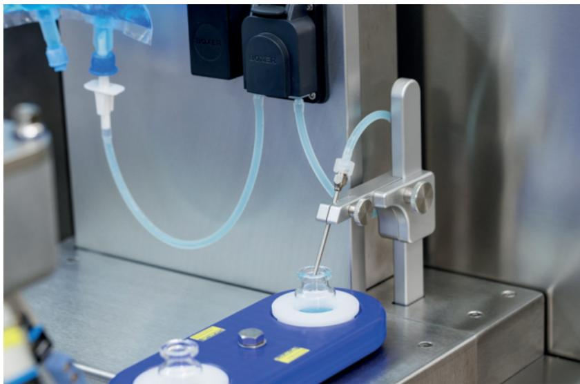
**Figure 3:** The dosing pump fills the injecting solution into the vials.
