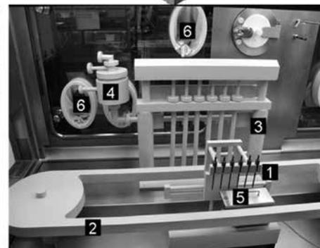
*Fig. 1: Experimental set-up with mock-up structure of a filling station (1) with conveyer (2), piston pump (3) and media reservoir (4) in the test isolator system. Position of the aerosol generator (5) is set at the filling station. Access to the production area of the isolator is achieved by glove ports (6).*
