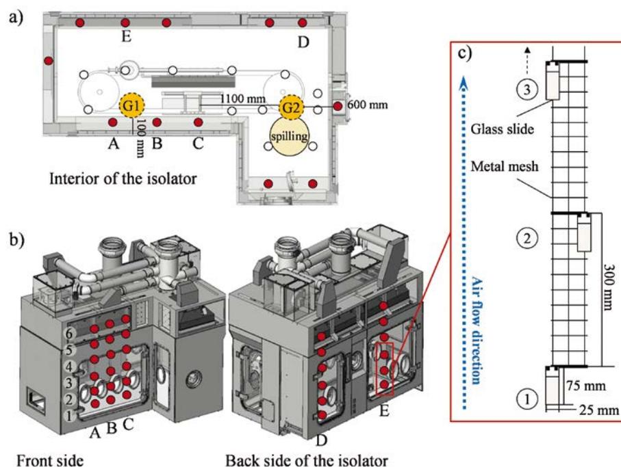
Fig. 2: Experimental set-up (a) with mock-up structure of a filling station and accordant sampling points in the production area of the isolator (white circles), aerosol generator positions (G1 and G2) and spilling area for handling failure. Red marked circles present sampling points at the bottom of the return air system. Figure 2 b) shows sample locations at return air system. Figure 2 c) demonstrates the sample fixation inside the return air duct.
