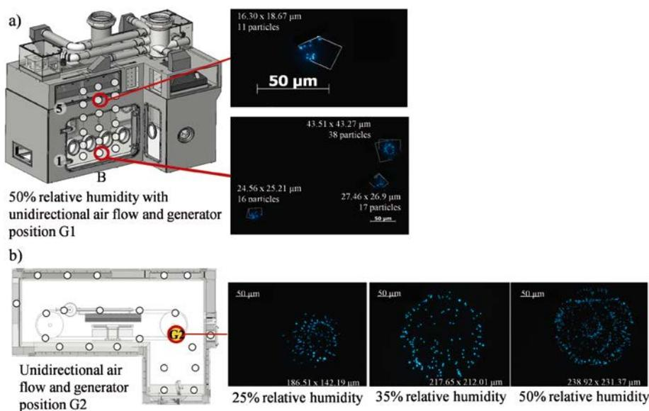
Fig. 3: Droplet size and particle number of aerosol deposition in the return air system, in dependency on distance from the generation source G1. (a); Droplet size in dependency on humidity at generation source G2. (b)
