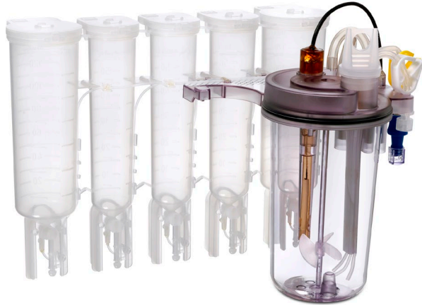
Figure 1: The new mini bioreactor unbaffled vessel design with a large pitched blade impeller, enables a gentle stirring and optimum growth of cell lines.
