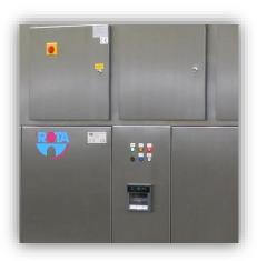
The high insulation grade of ROTA tunnels allows the electrical cabinet to be integrated, and consequently saves installation and maintenance costs of a separate dedicated room.
