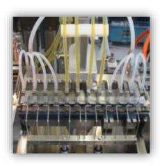
When processing ampoules, centering of necks at the filling and inert gas supply stations ensures the needles entering the ampoules in the centre position, thus wet necks and carbonised necks are avoided.
