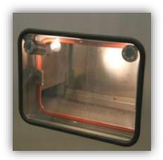
In addition to control windows in infeed and outfeed zones, ROTA tunnels feature a high grade of standard equipments like recorder, automatic shutter height regulation, automatic differential pressure compen-sation, chilled water air cooling... securing a perfect sterilisation and depyrogenisation process.
