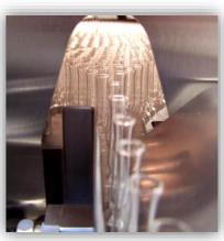
Once the containers went through all washing stations, they are turned by 180° in their outfeed position, released from the grippers and transferred with an outfeed scroll into the connected sterilisation tunnel
