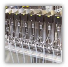
Filling generally happens using rotary piston pumps made of 316L stainless steel (ceramic also available) ranging from some microlitres to 125 ml, depending on the application and the machine. Other filling principles like peristaltic pumps or time-pressure may be delivered too.
