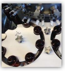
From the star wheel, the containers are picked up by suitable grippers mounted onto the central transport turret, turned by 180° and processed to the 8 inside and 4 outside standard available washing and air blowing stations.
