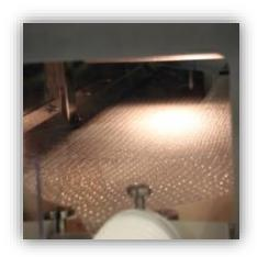
The containers are fed into the infeed zone of the hot air sterilisation and depyrogenisation tunnel, in which side belts ensure a perfect synchronisation with the washing machine.
